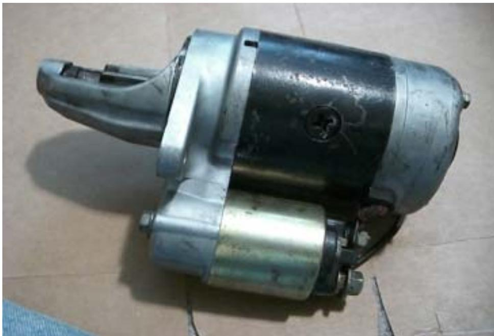
You will begin by removing the two circled bolts that retain the solenoid in place. You will not be using the solenoid so do as you will with it.
