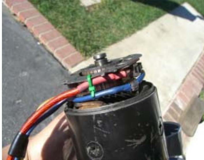
Once you have made certain that nothing is shorting out and that nothing gets in the way of any moving parts, re-assemble the starter by replacing the rear screws and bolts and the E clip. Make sure you can get all of the wires to exit the case. It's possible that you may need to drill a bigger hole to get all of the wires through.
