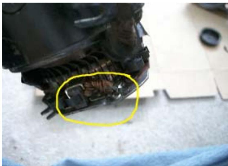
Most starters that have not had anything done to them will have two of the brushes contacts tacked together to the field magnet coils instead of being soldered together, as is the case with this particular starter.
