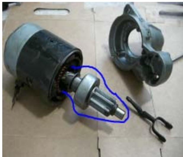
Next remove the brushes from the rear cover by removing the two phillips screws on the rear. you will also need to remove the plastic cover (arrow) because there is an E clip underneath holding the rotor in place.
