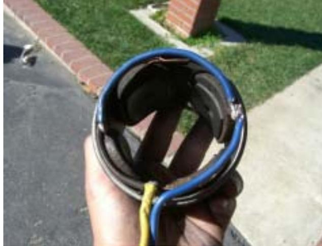
Next, I soldered a red piece of 10 gauge wire to one of the brushes that originally lead to the field coils. The yellow line will be where a second piece of wire will attach to the brush on the opposite side of this one. You will want to protect these wires with some heat shrink so that they're not touching anything else. You will probably want to do the same with the field coil wires.
