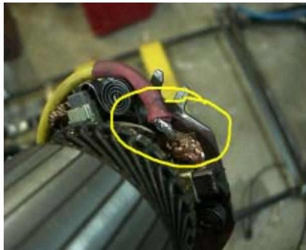
Once you solder all the wires into place, assemble the brush plate with the rotor and the field coils together to see how they will fit and to make sure that none of the contacts short out with each other. Make sure that none of the cables will be getting in the way of any moving parts. This picture does not show the yellow wire running to the second brush because it was taken prior to me soldering the other wire into place. I was trying a little experiment which failed.
