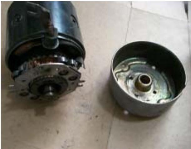
As we can see, there is electrical tape on some of the conductors inside this motor, which leads me to believe that this is a remanufactured unit and that could be the reason why it was so clean looking to begin with! the conductors underneath the tape will need to be separated from each other as I will show later on.
