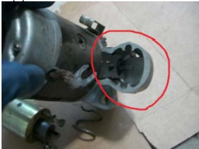
Next, you will focus on the rear end of the starter and remove the two long bolts that hold the whole thing together. These are circled in red.
